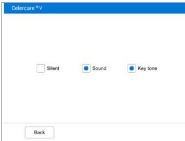
2. The user can select **‘Sound’**, **‘Silent’**, or **‘Key Tone’**. **‘Sound’** refers to the prompt tone when opening the analyzer and completing the analysis. **‘Key Tone’** is the prompt tone for pressing buttons.
