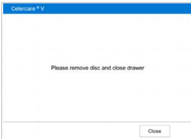
11. Press 'Open' to access the drawer and remove the disc. Afterward, press 'Close' to shut the drawer and return to the main screen. The analyzer is now ready for another test.
