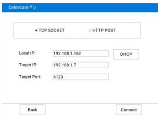
2. After selecting the communication method as '**TCP SOCKET**' or '**HTTP POST**' the '**Device IP**' will be displayed automatically. The LIS engineer will then enter the '**Target IP**' and '**Target Port Number**' which refer to the IP address and port of the LIS server.
