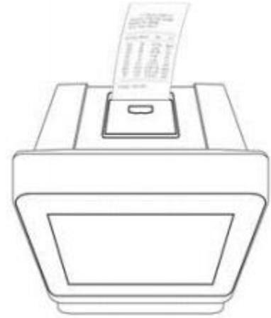
***Note: After installation, the thermal side of the paper must face down. If installed incorrectly, it will not print reports. (Some models do not have a built-in printer.)***
