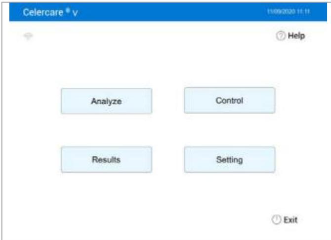
1. On the Main screen, press 'Control' Controls can be accessed at any time while the analyzer is displaying the Main screen.
